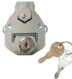
7461 Medium surface mount twist latch, keylockable. Meterail: steel Size: 73.5*65.8mm Finish: zinc/chrome
